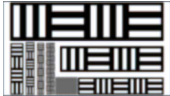
Resolv4K Zoom @ 4.5X High Mag 8.9MP Sensor – 0.76µm / pixel 3.56mm FOV – 5.20mm 2 Area (3.25X more)
