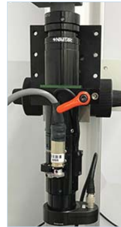
Optotune Module (Navitar 1-64805) with Zoom 6000 Motorized System
